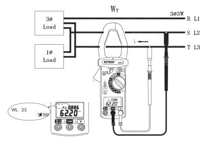
3. The power clamp will process these two sets of data ( $W_{L12}$ ,  $W_{L23}$ ), and show the result on the LCD. The  $W_{L123}$  symbol will be shown to indicate  $3_{\varphi}3W$  power. The  $3_{\varphi}3W$  power (in watts) is stored in the meter memory.
