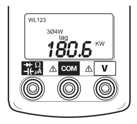
To read a single data record, use the "HOLD" key to select WL1, WL2, WL3 or WL123 display then press the "RANGE" key to select KW+HP (Horse Power), KW+PF (Power Factor), KW+KVAR, KVA+ $\theta$  (Phase Angle) or A+V displays.
