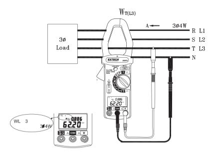
4. The power clamp will process these three sets of data ( $W_{L1}$ ,  $W_{L2}$ ,  $W_{L3}$ ) and show the result on the LCD. The WL<sub>123</sub> symbol will be shown to indicate the  $3_{\varphi}4W$  power (refer to diagram).
